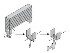
Attach the counterweight support bracket to the frame by placing the flat washer over the 13 mm • 1/2 in bolt and running the bolt up through the bracket and the frame. Then place the lock washer on the bolt. Secure the bolt with two nuts. Repeat with the other bolt.
