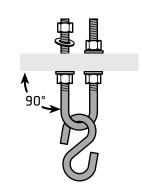
The Pullout Switch should be installed near the U-bolt. If the S-hook is activated, the cable will pull the key downward and trigger the switch.
