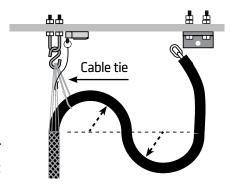
Once positioned, secure the bottom of the mesh grip to the cable with at least 4 wraps of electrical tape. Make sure that the safety loop does not get caught on any pit equipment (ex: car buffer).
