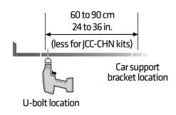
Attach the car support bracket to the bottom of the car frame as shown.
