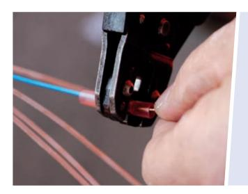
Both stripped core ends are connected with a crimp splice and joined together with a pincer to be tension-proof.
