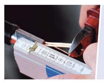
The shielding wires are also shortened according to instructions.
