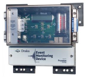
The DRK-S701-ROHS EMD detects and measures seismic events and signals elevator controls to take appropriate action based on their magnitude.
