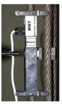
metric units for up to 12 ropes. The clearly displayed tension information allows the field technician to quickly and accurately equalize the rope tensions. Since the information is displayed in real time for each rope, the impact of a tensioning adjustment made to one rope is immediately visible on the other ropes.
